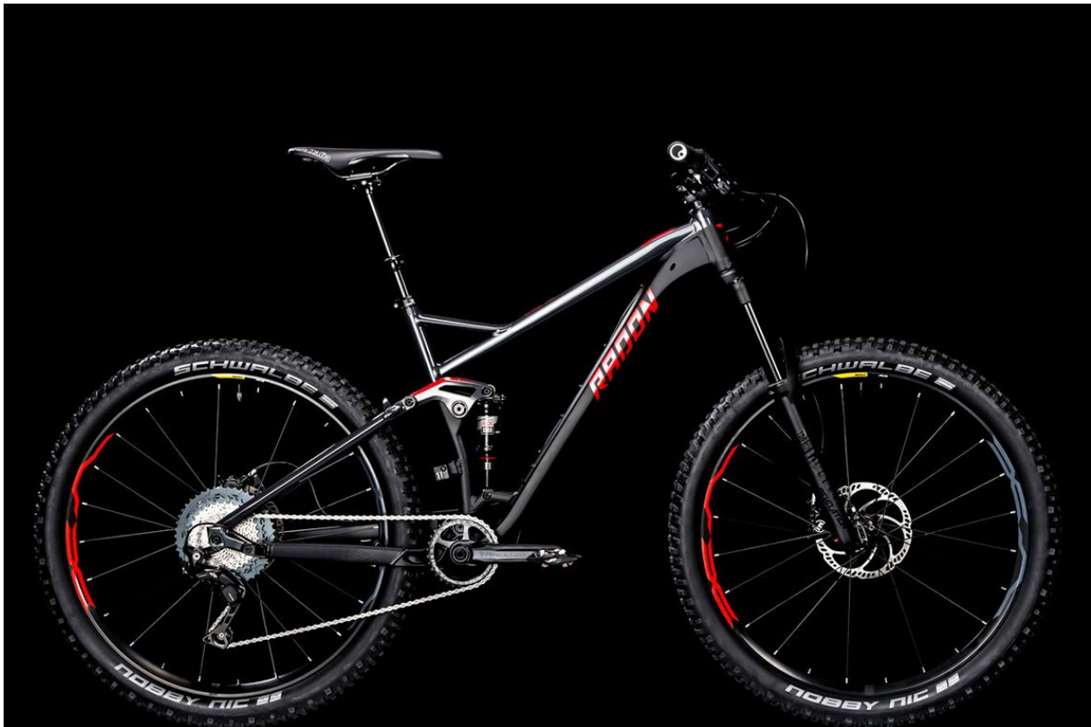
Radon Slide in 27,5+ (650B) Federweg: vorne 150mm, hinten 140mm
